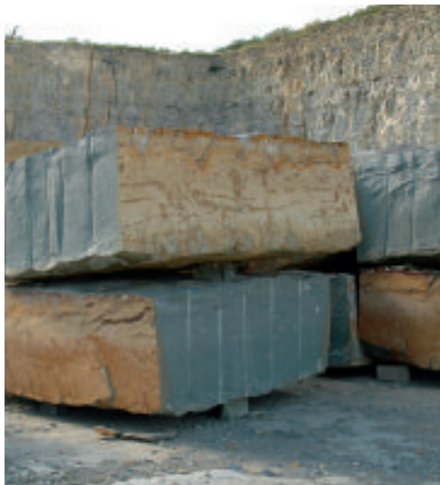
During the manufacture of natural stone slabs, raw blocks from the quarry are sawed into 4 cm-thick panels
